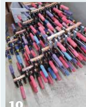
10 The author typically glues up thirty pen blanks at once to improve efficiency. The veneer strips are glued in one at a time, as the glue must be allowed to dry before proceeding to the next curvy cut.
