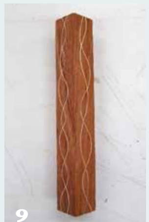
9 A pen blank with four strips of veneer glued in on two planes, ready for turning.
