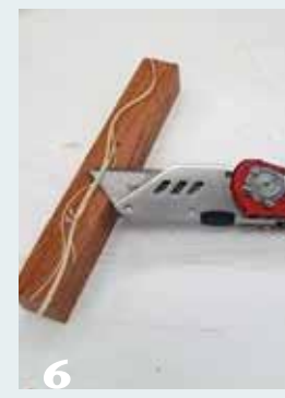
6 A sharp utility knife makes quick work of trimming any veneer standing proud of the blank.
