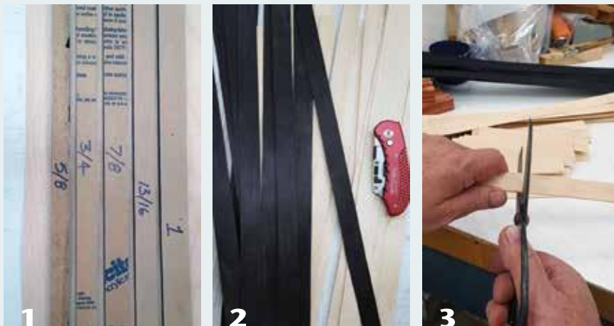
1 Strips of sheet acrylic precut and labeled at defined widths to accommodate various pen blank sizes. These templates act as a fence when cutting the veneer with a sharp utility knife.
