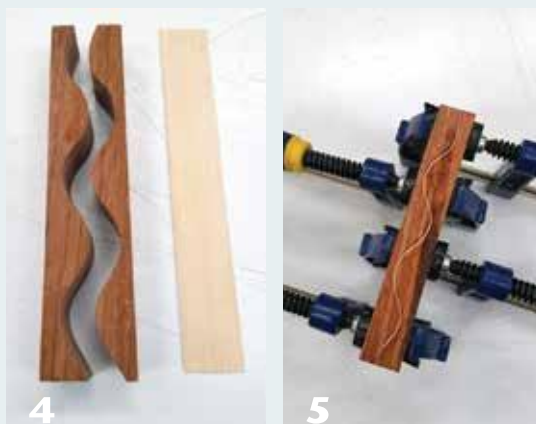
4 Cut a curvy line along the length of a pen blank, then glue in a contrasting strip of veneer. Begin clamping in the middle and work outward.
