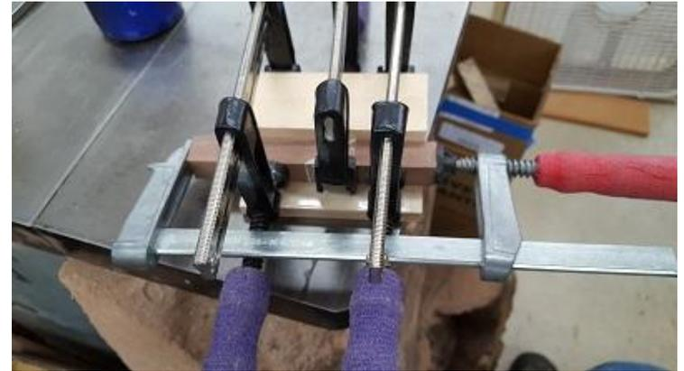
My clamping fixture is a piece of construction lumber with packing tape to prevent the glue from sticking.
