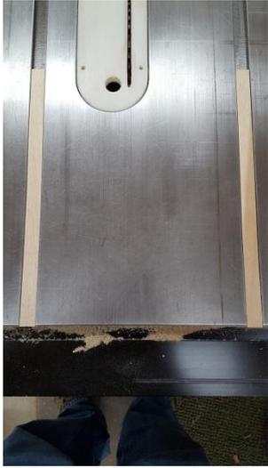
Start by cutting 2 strips to fit into your table saw slots. Should be a snug fit but not tight. The thickness of the strips should be less than the depth of the table saw slot. You want the board of the jig in contact with the saw surface.
