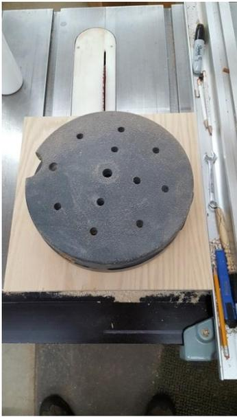
Cut a board approx 18" square. Spread glue on the strips. Lay your board on the strips and weight down until the glue sets. I lined the strips up with the edge of the table and the board against the rip fence. You don't have to do that, its just the anal engineer in me.
