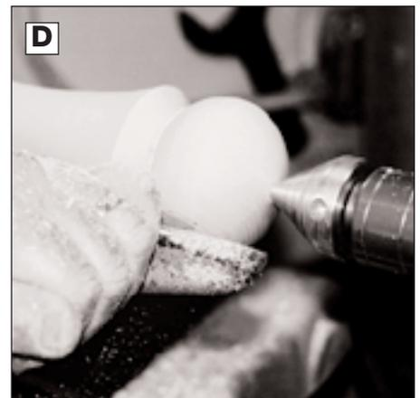
end. Turn a 1" tenon approximately  $\frac{1}{2}$ " long on the bottom end of the cap, then make a finishing cut from the perimeter toward the tenon. The tenon will fit into the 1" through hole in the
