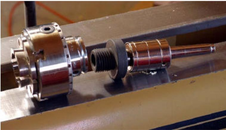
Reverse chucks give you many options for turning the bottom of your bowls, vessels and platters. Here are some examples of what you can do with reverse chucks.
