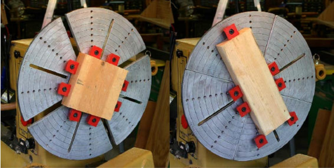
One disadvantage of these chuck jaws is the wrench. They don't come with an extended wrench to tight the jaws and the T wrench that comes with the chuck won't work to tighten the jaws. I have these installed on a Vicmarc chuck which uses a standard allen head. You could easily use a ball end allen wrench on this chuck but I simply welded an allen wrench onto a longer rod so the T handle would clear the jaws.
