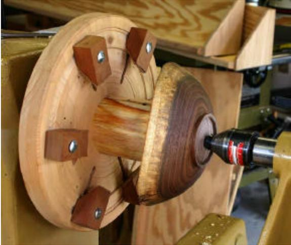
Because the jaws are independently adjustable you can hold square or oblong pieces to turn the bottom. Here is a photo of a natural edge bowl being driven by friction with the extended jig attached to this chuck.
