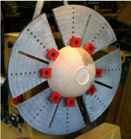
Because the buttons are easily positioned in different holes you can hold odd shaped piece for turning.
