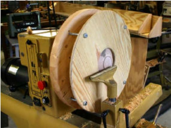
The bolts can be a little dangerous. To limit the problems I use all thread rod and extend as much rod as I can through the back of the chuck. This keeps the rod out of my turning area. You can also reverse turn hollow vessels with this system. Simply replace the bowl turning all thread with longer pieces to accommodate the hollow vessel.
