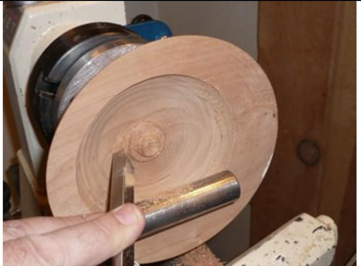
After completing the hollowing of the bowl, the rim of the bowl is wider on one side than the other. Sand the inside of the bowl before readjusting the chuck back to center.
