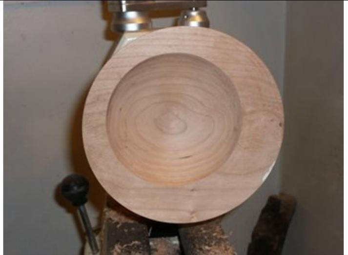
Reverse mount the bowl so the glue block can be turned off. I use a set of Nova Mini Cole Jaws to hold it. After the glue block is gone, the foot of the bowl can be finish turned and sanded.
