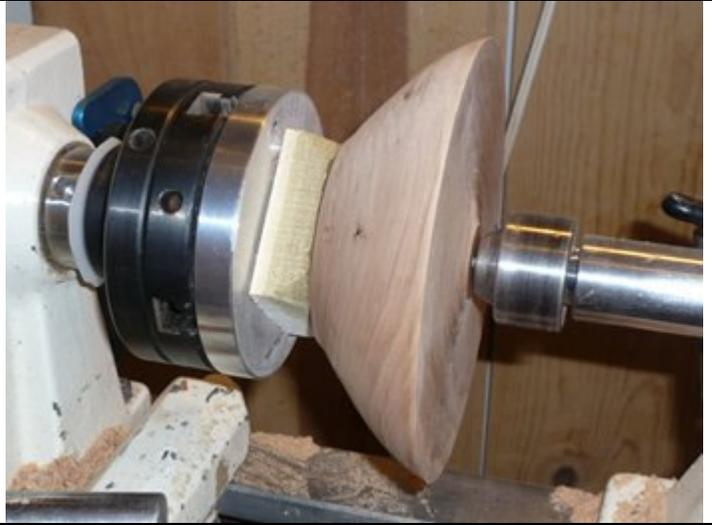
After completing the shaping of the outside, loosen the screw in the slot and move the plate to its off-center position. My chuck allows for an approximate 1/2" offset.
