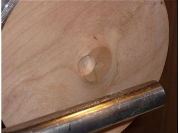
The inside of the bowl is hollowed out in exactly the same manner as any other bowl. The only differences are that there is an off-balance rotation and the wall does not have the same thickness all the way around. To handle the off-balance rotation, the speed of the lathe needs to be adjusted to ensure that the vibration doesn't cause problems.
