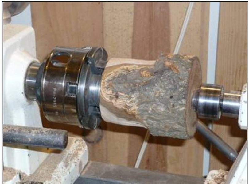
At this time, I start to roughly shape the blank into the form I want to turn. I usually look at the grain of the wood to help me design the form I want to use. I leave approximately 1" of wood between the form and the chuck. This is to ensure that I have enough wood to make a jam chuck for finishing the bottom.
