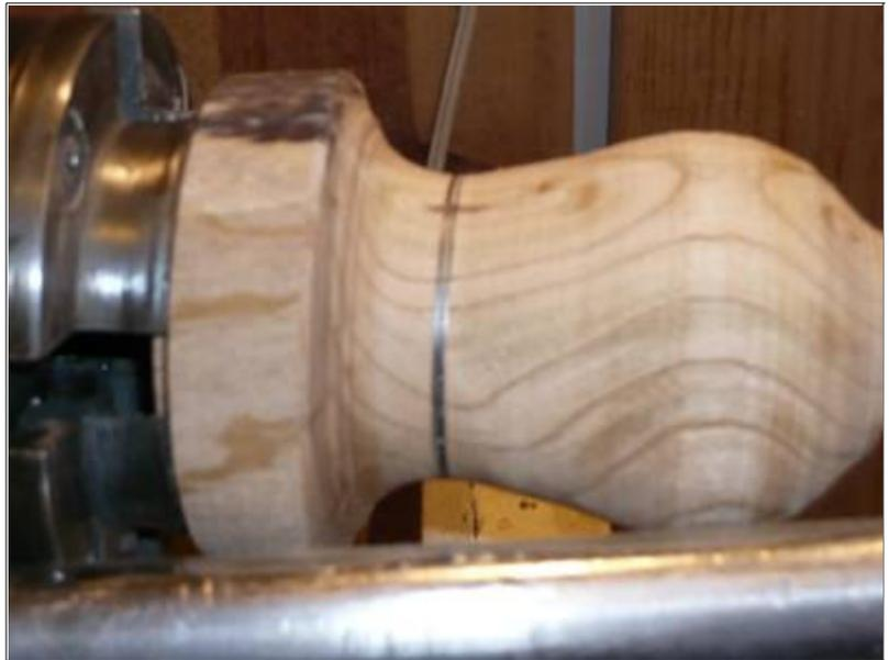
Now, it's time to start hollowing. My favorite tools to use are the min- Kelton hollowers, but any hollowing tool will work. It is just a matter of preference. I will remove the tailstock from the lathe and position the toolrest across the opening in the form.
