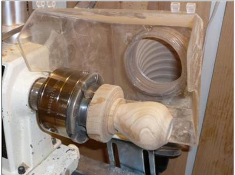
To finish the bottom, I turn a jam chuck from the remainder of the stock that is still in the chuck. This takes the form of a small tenon that is about  $\frac{3}{4}$ " in diameter. The opening in the top of the form should fit tight so it doesn't slip, but not so tight that it cracks the lip. I use a piece of paper towel on the tenon if the fit is too loose.
