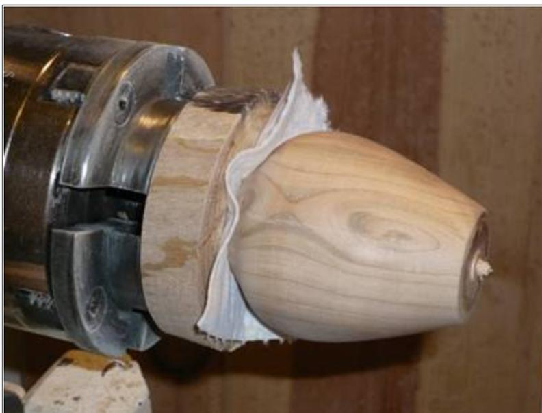
Once the reversed form is centered on the jam chuck, I use my dremel with a 120 grit drum to do the initial sanding and shaping of the foot.
