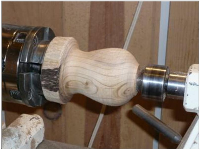
Using a  $\frac{3}{4}$ " forstner bit in a drill chuck mounted in the tailstock, I drill a 2" hole into the blank. With a pencil mark a line on the outside of the roughed form. This line will be an indicator so I know where the foot will be.
