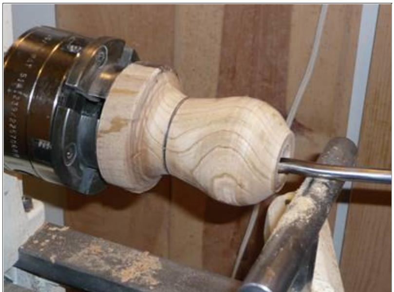
Hollow the form, clearing the shavings often, and checking the wall thickness for uniform thickness
