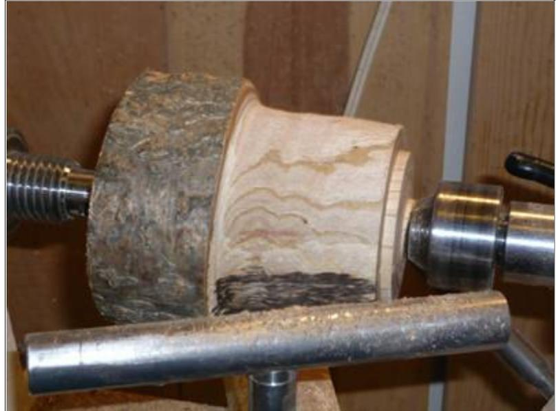
I then remove the blank from the centers and mount it in my chuck. I pull up the tailstock for extra support.
