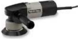
Don't be afraid to use the coarser grits sandpaper. Better to start with a 60 or 80 grit sandpaper and move up from there than to over-sand with 220 grit. When you feel a wavy bowl, it frequently is a sign of over-sanding. The softer wood is abraded away more rapidly than the harder growth rings, leaving a waving surface. Using a larger sanding disk with a hard backing helps to minimize this problem.
