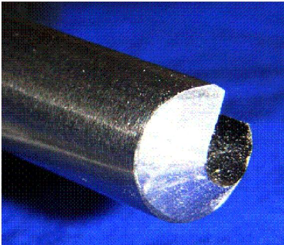
Many turners will tackle tear out by changing to a gouge with a steeper angle than the 60 degree Ellsworth grind. They go back to the older angle of 40-45 degrees. This is the principal behind the Hout gouge and the finishing gouge sold by Trent Bosch. I am beginning master the use of the Bosch finish grind and it produce good results.
