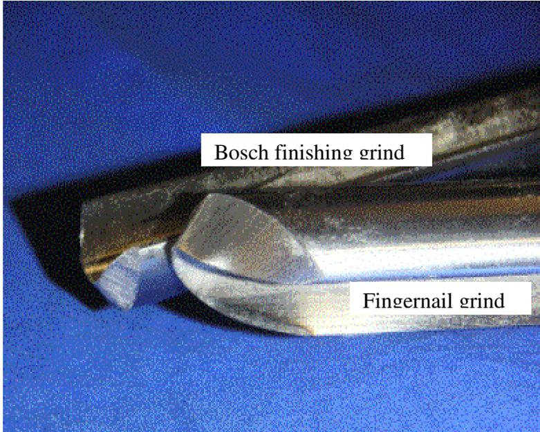
Gouges – my experience is that a shearing cut on a sharp gouge is the best way to clean up tearout. This can be a bit difficult to describe, but here goes – the shearing cut inside a bowl is achieved by rubbing the bevel and using the left side of the gouge near the tip as the cutting edge. This works rather easily if the gouge is properly shaped as a classic Ellsworth grind.
