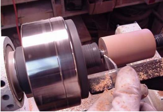
Remove the blank from the mandrel again. With a hand chamfer tool, bench knife or pocket knife clean up the edge around the hole. Put the sizing ring back in place and thread the blank on for the last time. The preparation steps are complete and you can begin to turn your design on the stopper. I find it helpful to keep the tail center in position as long as possible. It reduces vibration and allows much more aggressive cutting during the early stages of turning the shape.
