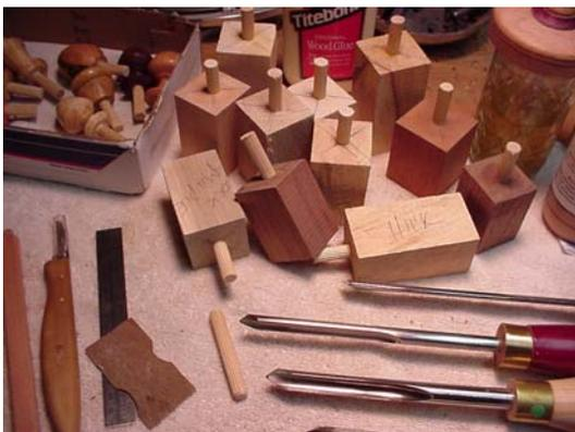
Next mount the blank in a 3/8 dowel chuck. A dowel chuck is a drill chuck but the jaws have been bored out to fit the 3/8 dowel. This prevents crushing the dowel which definitely will cause an off center situation and may weaken the dowel enough to create a safety hazard. I do know a turner who uses his 1/2 drill chuck but protects the dowel with a split piece of copper pipe. Even with the dowel chuck be careful not to overtighten.
