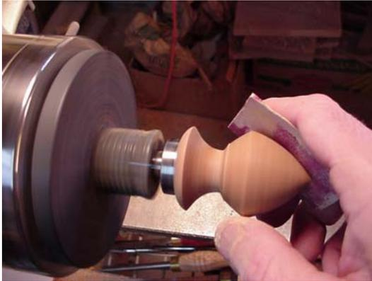
Before finishing you may want to burn a line or with the tip of your skew add a few tiny lines. In the photo below I am burning a small reveal under the globe of the stopper design. I find a business card sized piece of HPL or Formica to be very effective and safe for this task. Color sample cards are an excellent free source of laminate for burning. You can sharpen the edge to get the size line you wish. Wider lines can be friction burnt with Masonite or tempered hardboard.
