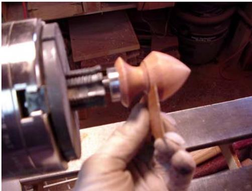
I use two finishes on Stoppers. On natural woods I will first brush on a thick coat of Deft which I buff dry with a paper towel on a fast running lathe. Thin the Deft with Lacquer thinner about 50/50. The Deft acts as a sealer and I find it easier and more versatile in my shop than other sealers. On top of the Deft I put a couple coats of Myland's Friction Polish. Myland's Polish takes a little more care to apply than HUT Crystal Coat but I think it lasts longer.
