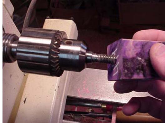
Bring your tailstock up into position and bring the blank to nearly round. A medium sized roughing gouge and big bowl gouge is very effective for 'banging' the part round. My 3/8" bowl gouge is a favorite when turning stabilized blanks. Once you get to 90% round stop the lathe and look for cracks, splits or voids that may be of concern to your design or safety. A little CA can save most mildly split blanks or create a design that will remove the bad area of the blank.
