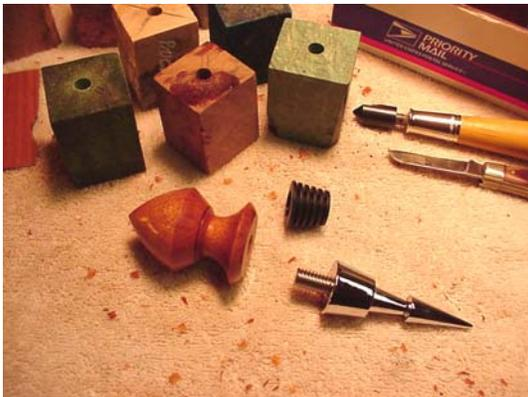
After assembling the hardware you may choose to wax the stopper and the chrome hardware. Renaissance Wax is excellent but a standard wax like clear Briwax is fine. After applying the wax wait a few minutes and buff it with a paper towel. Viva brand towels have no quilting and leave no lines when buffing. I would like to try a Beale Buffing system on the stabilized stoppers but haven't made that investment yet.
