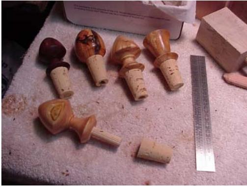
Put a dab of PVA adhesive on dowel. Slide the cork up the dowel giving it a few rotations to spread the glue. It does not take much glue. Wipe off any adhesive that squeezes out.
