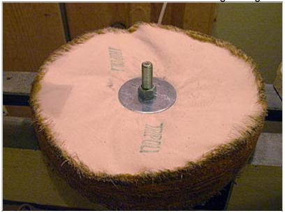
The thread on the bolt screws right into the chuck.
