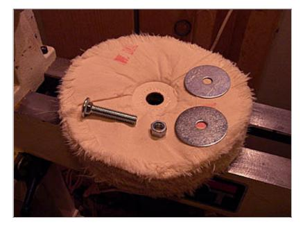
I assembled them with a washer on each side and the bolt running through with the nut tightened.
